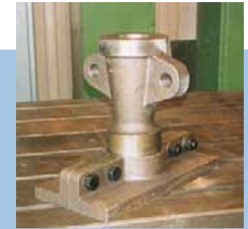
Spherically seated rope gland Designed & Manufactured for Hatfield Colliery
