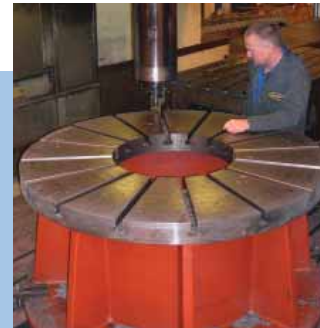
1800mm dia cast iron machine fixture Design & Manufacture Stephenson Engineering
