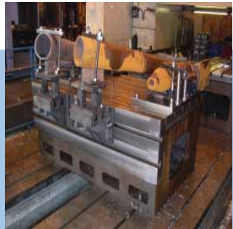
Five ton cast iron machine table Design & Manufacture Stephenson Engineering
